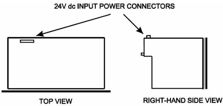
Redundant +24Vdc power is supplied to a plug connector at the rear top of the chassis, as shown in Figure 5-2. Redundant power is supplied to all modules in the chassis through the backplane.
